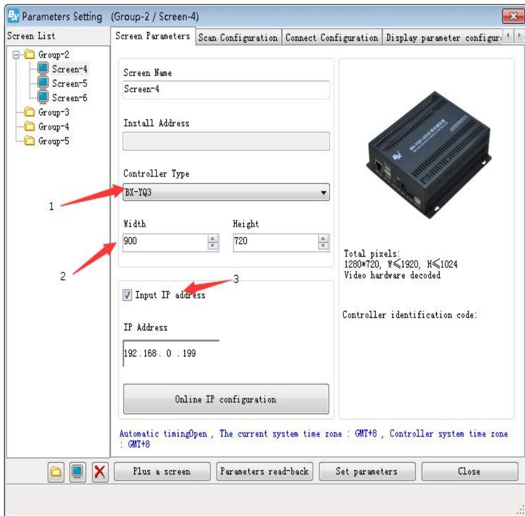
Step 1: Select the correct controller model, usually, if your connection is right, the PC software could identify the controller model automatically, under this circumstance, you do not need to select manually. please choice BX-YQ3 if you are using BX-YQ3
