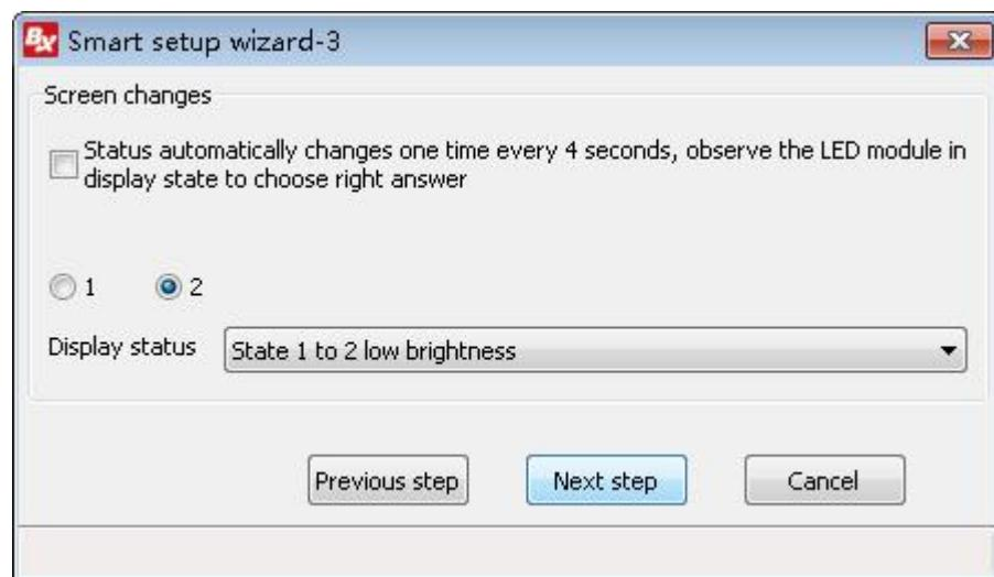
Select the correct display status, click "next step", enter into "Smart setup wizard-4", check the picture below:
