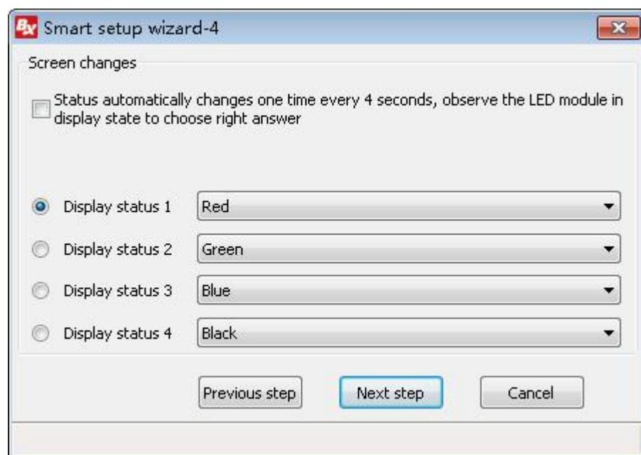
Select the correct display status, click "next step", enter into "Smart setup wizard-5", check the picture below:
