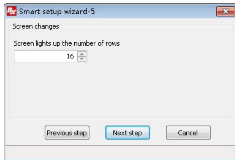
Select the correct display status, click "next step", enter into "Smart setup wizard-6", check the picture below:
