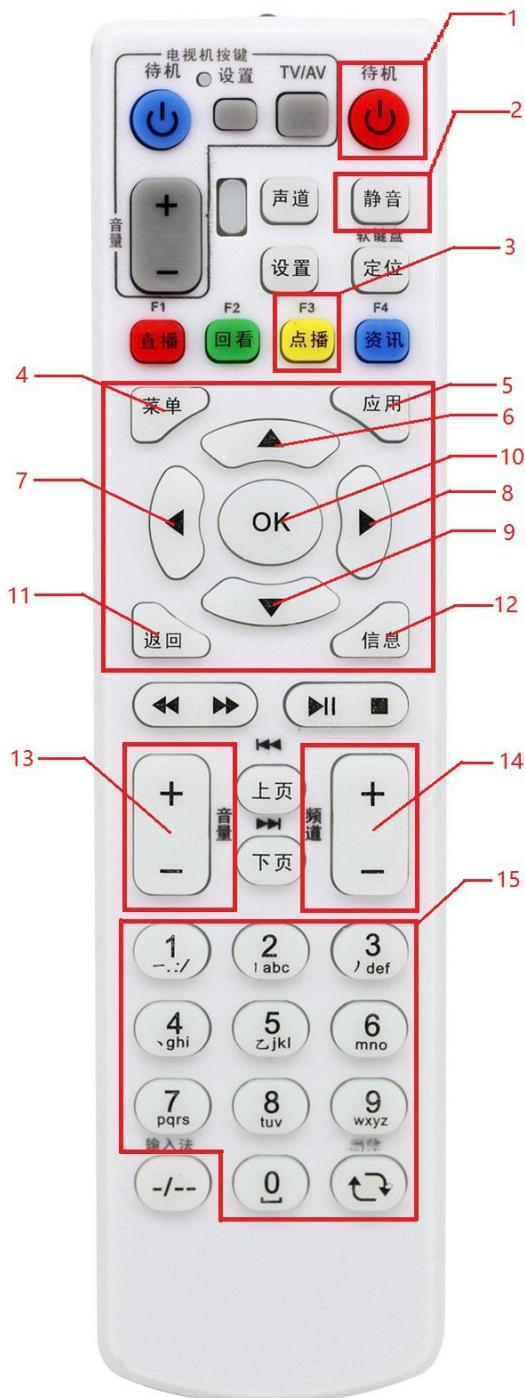
ZTE Set-top box remote controller, the buttons marked in red can be used for ONBON controllers ;
