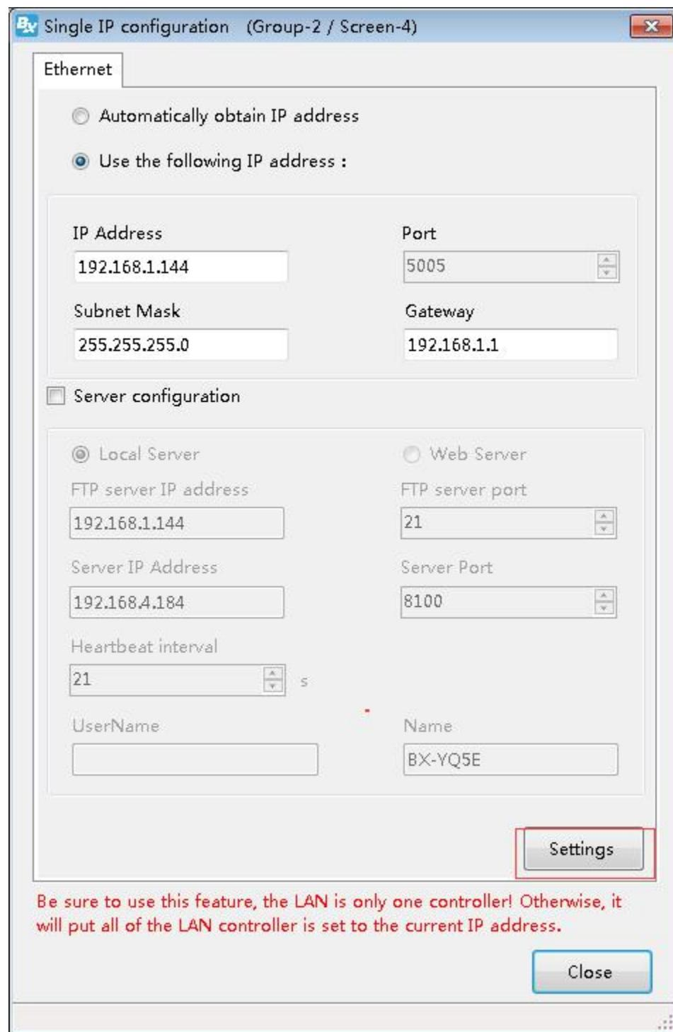
The default IP of controller is "192.168.0.199". If it's by direct link, without router, then, the IP of controller and PC should be on the same network, or it will be failed. And if it's failed because of the IP setting, then reset IP address, it will get OK.
