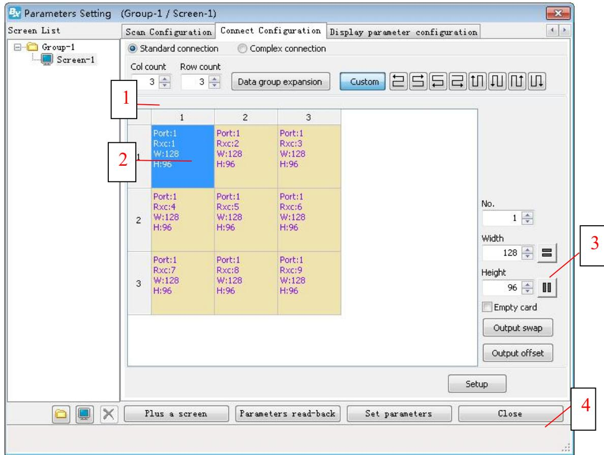
Step 1: Input the correct cards quantity horizontally and vertically according the actual quantity you use on the screen;
